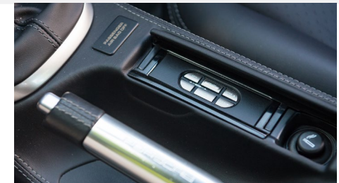
An alternate custom-install of control unit
