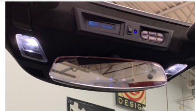
Custom Radar-View pod designed for a 2018 convertible Corvette ZR1
